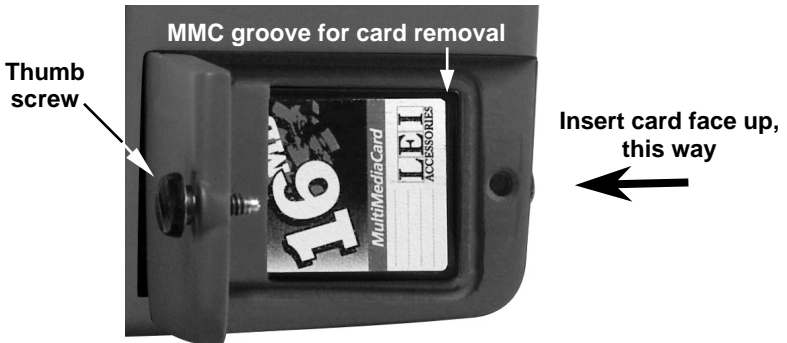
Memory card compartment with a 16 MB MMC card installed.
